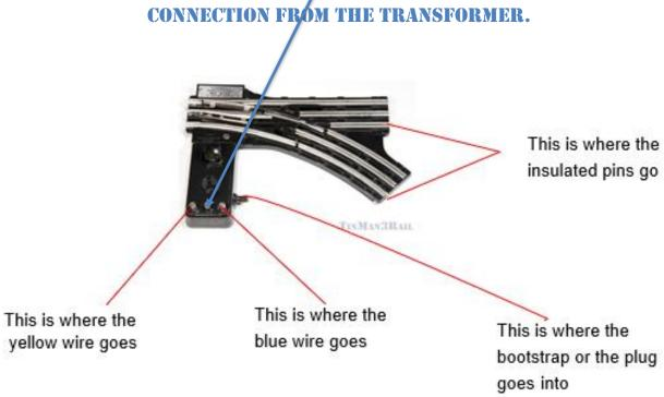
THE RED WIRE FROM THE 8' CABLE GOES TO THE RED WIRE FROM THE BOOTSTRAP PLUG, THE BLACK TO THE BLACK WIRE
